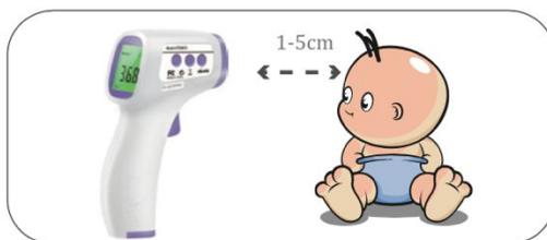
Figure 2: Measuring position and distance
